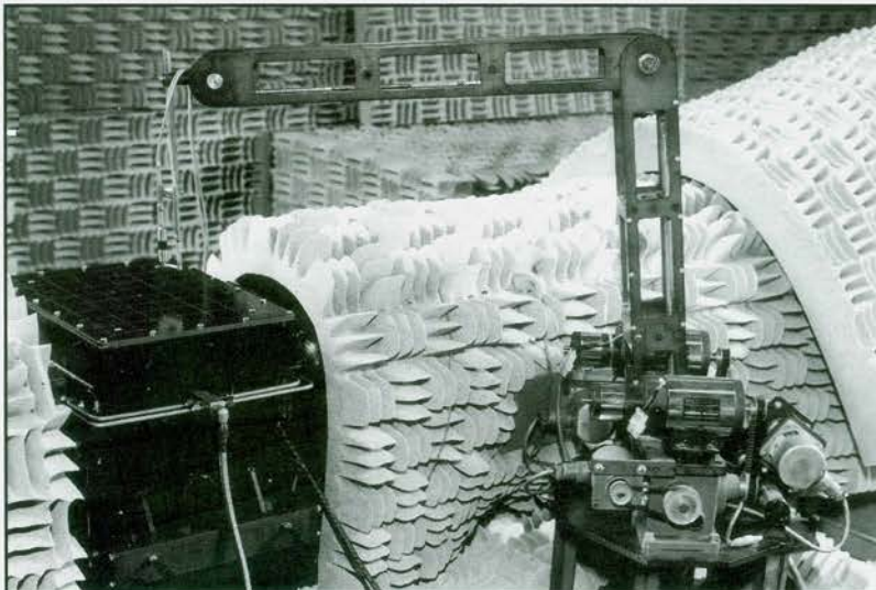
Fig. 3 — Test gearbox and RAIMS robot.
