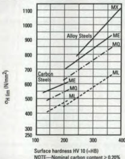
Fig. 2 — Through hardening steels: Allowable stress numbers (contact).
