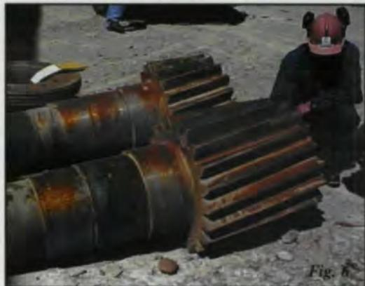
Fig. 6—Failed pinion removed from #2 ball mill in August 1998.
