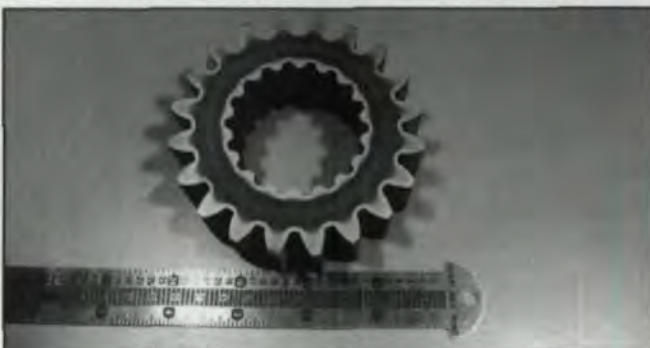
Fig. 9—An induction heat treated gear made from specialty TSH steel.
