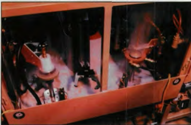
Fig. 7—Induction heat treating an automotive transmission gear with internal and external teeth.
