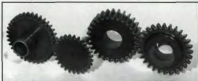
Fig. 1—Sample induction hardened gears.
