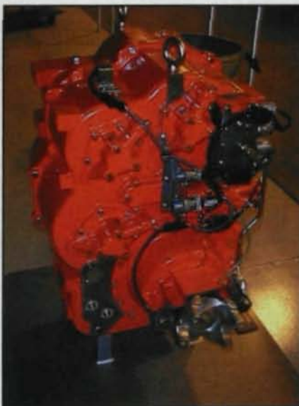
Fig. 1 — These Twin Disc transmissions incorporate 14 to 16 large gears like the one shown above at right. The six-pitch helical gear is for one of the three 205 mm (8 in.) clutch pack assemblies in a TD-61-1175 transmission (right). The SAE 8620RH gear is carburized to 0.81 mm (0.032 in.) min. finished effective case depth at 60 to 64 HRC surface hardness. The TD-61-1175 transmission is used in airport crash-fire vehicles. It's rated at 400 kW (540 hp) at 2,300 max. rpm. The 2600 series transmission, above, is used in Versatile 1150 series tractors. It's rated at 520 kW (700 hp) at 2,200 max. rpm. Photos courtesy Twin Disc Inc.
