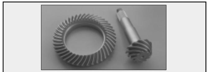
Figure 11—Ring gear and drive pinion.
