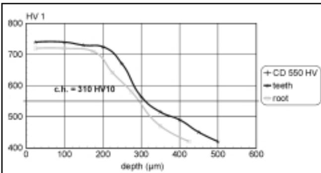
Figure 15—Hardness profile of smaller 16MnCr5 gear wheel.
