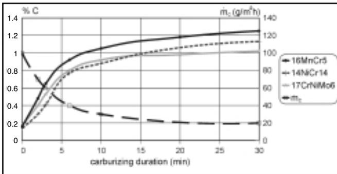
Figure 2—Surface content of carbon vs. carburizing duration.
