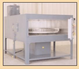
1/4 hp motor through a gear reducer with a torque limiting device. The hearth indexes one position each time the loading door is opened or closed.
