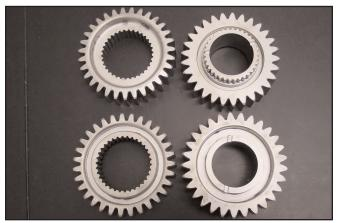
Figure 4—Racing transmission gear (AISI 9310).
