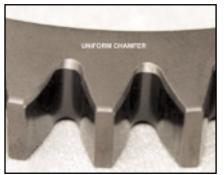
Figure 6—Uniform chamfer as produced by chamfer hob.
