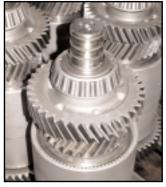
Figure 1—Fire truck transmission gears. (Photograph courtesy of Twin Disc Inc.)
