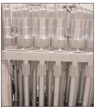
Figure 7—Racing transmission main shaft (AISI 4820).
