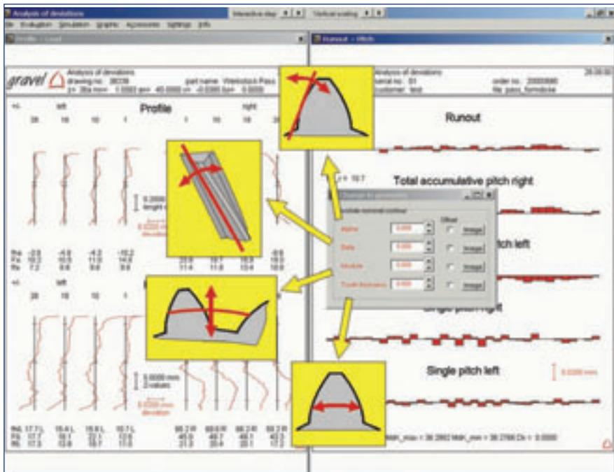
Figure 8—Program for the analysis of gear deviations.
