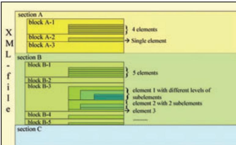
Figure 4—Flexible structure design of an XML file.
