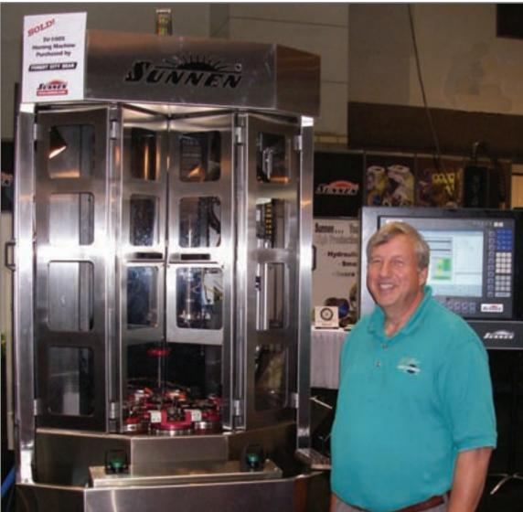
fully automated vertical machine—uses Sunnen's patented Krossgrinding® tools, which the manufacturer says are capable of controlling bore size down to 0.00005" and finish to 16 µin or better.
