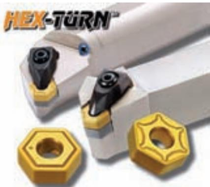
finish, even at high feed rates. The 45° lead angle allows high feed rates with low cutting forces. A 120° included angle provides a strong insert design and improved resistance against notching.
