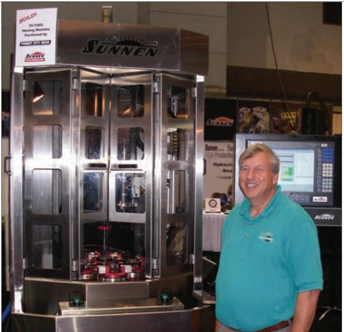
fully automated vertical machine—uses Sunnen's patented Krossgrinding® tools, which the manufacturer says are capable of controlling bore size down to 0.00005" and finish to 16 µin or better.
