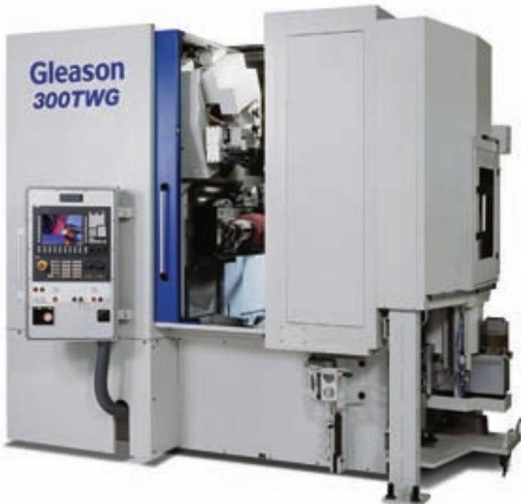
The 300 TWG from Gleason Corp. is designed to deliver fast floor-to-floor times for grinding of cylindrical gears with a diameter up to 300 mm.
