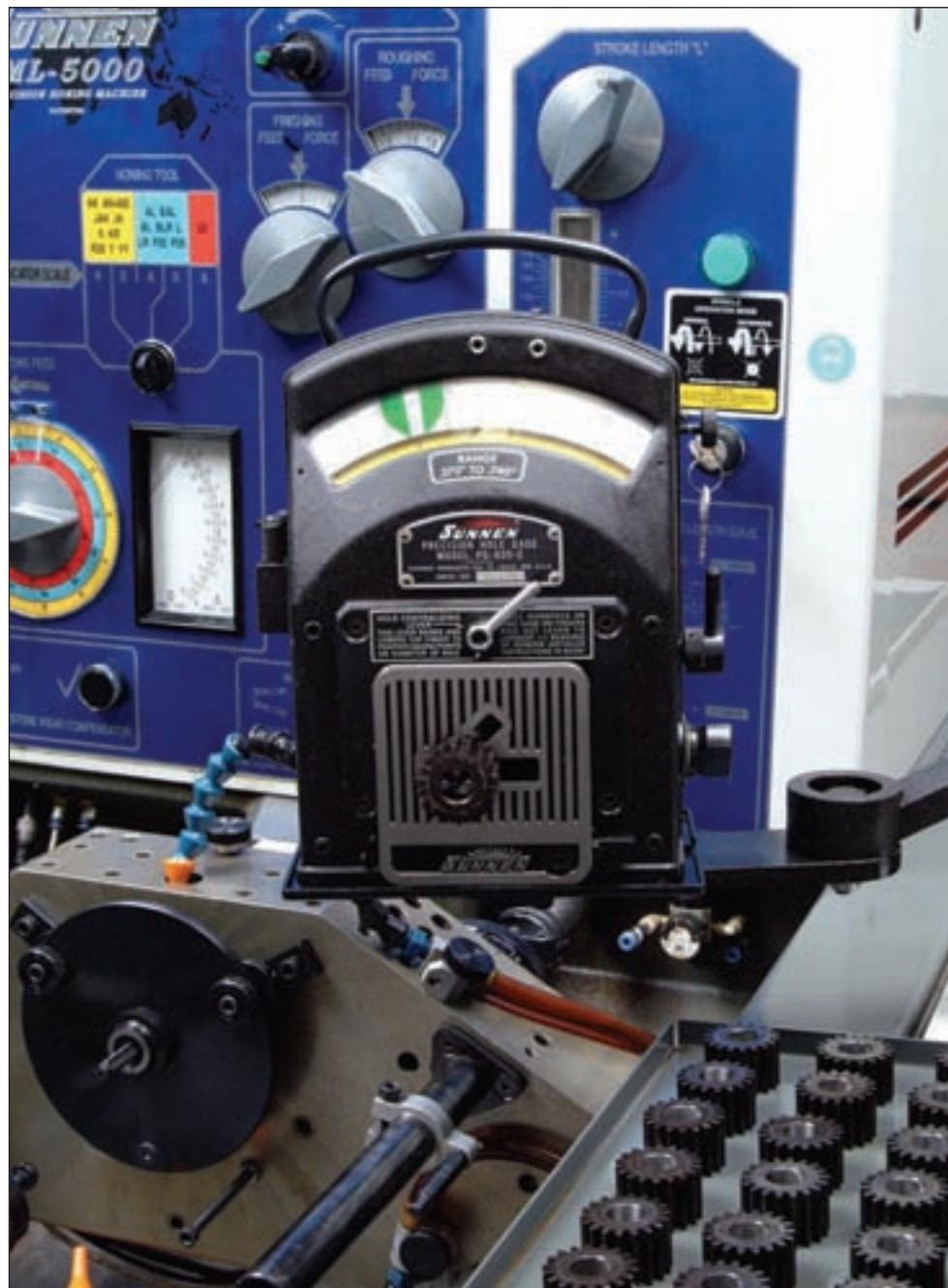
helps to eliminate friction and wear to maintain repeatability and linearity, no matter the gage's age or amount of use. A PC-Series bore gage system comes standard with everything needed to measure any bore size in its range. Accessories are available for special requirements.
