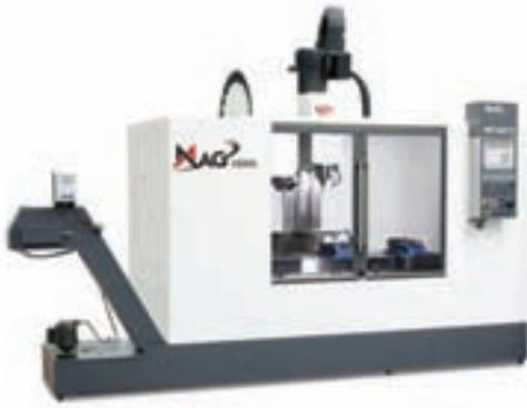
Both versions feature box-way construction with integral flame-hardened ways complemented by Steinmeyer ETA+ dual-mounted ball screws. Rapid traverse is 1,000 inches per minute with a cutting feed rate up to 800 inches per minute.
