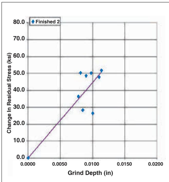
Figure 21—Change in the longitudinal component of residual stress as a function of grind depth for gear Finished 2.
