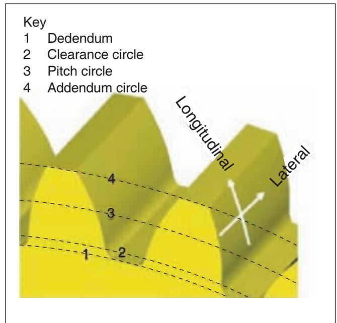
Figure 2—Longitudinal and lateral tooth directions on tooth.
