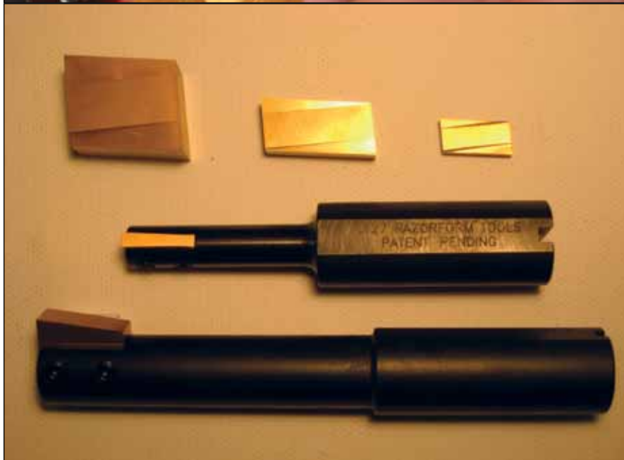
Razorform Tools carbide inserts remain in the machine turret during indexing, resulting in longer tool life while reducing downtime.
