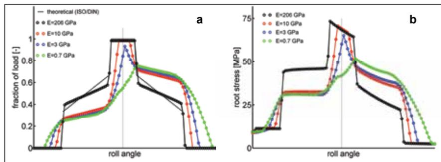
**Figure 1—(a) load sharing and (b) root stresses as function of roll angle for a steel pinion and a steel gear (black circles), a glass-fiber (GF) reinforced-plastic gear (red circles), an unfilled plastic gear (blue circles) and an unfilled plastic gear at elevated temperature (green circles). The dashed black line is the load sharing according to (steel) theory (ISO 6336) and the dotted black line represents the pitch point.**
