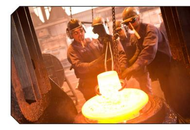
"The process looks very simple," Kantus said of Ajax's method of making rolled rings. "We start out with bar material and we cut it to a weight, and then we forge it into a pre-form so it looks like a donut. That then goes on a rolling mill where you can roll it out to the required dimensions. Then most of them go to heat treat and then machining.
