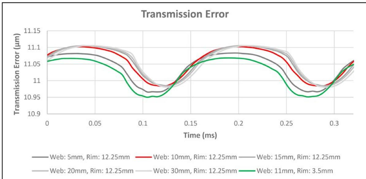
Figure 14 Transmission error for different gear blank dimensions.
