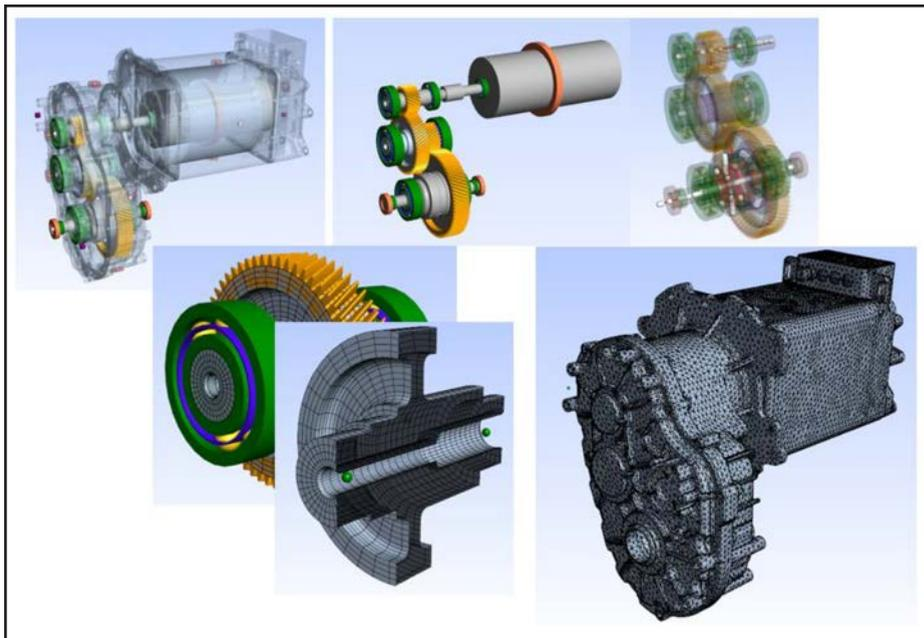
Figure 4 FE-based bespoke EV system analysis model.
