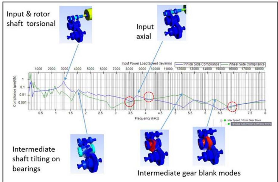
Figure 6 Gear blank mode influence on wheel-side compliance.
