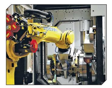
The end-of-arm tooling consists of multiple grippers. Each gripper has three Gleason-designed gripper fingers which apply frictional forces to grip the part firmly and accurately. The gripper fingers accommodate a wide range of parts, saving change-over time. When necessary, the gripper fingers can easily be replaced.
