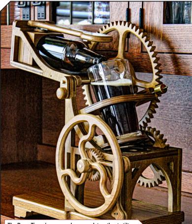
The Brew Tipper's gears and cam work together to tilt a beer bottle forward and tilt a glass backward so beer runs down the inside of the glass, which keeps the beer from getting too foamy. (Photo courtesy of Clayton Boyer)
