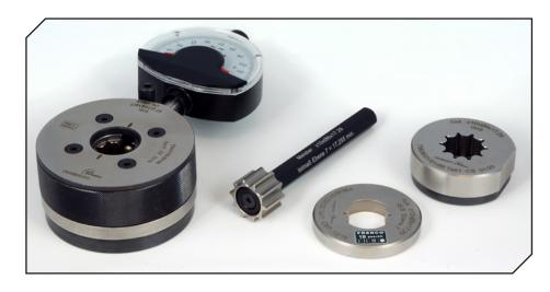
shaft must not exceed the end surface of the Nogo ring gage.
