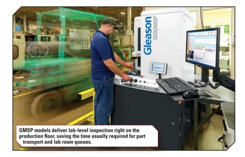
production machines in a Closed Loop, so program corrections can be made at the machine tool real time.
