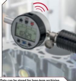
Data can be stored for long-term archiving, recording when the part was measured and by whom. It can also be used for tracking and improving operator throughput.
