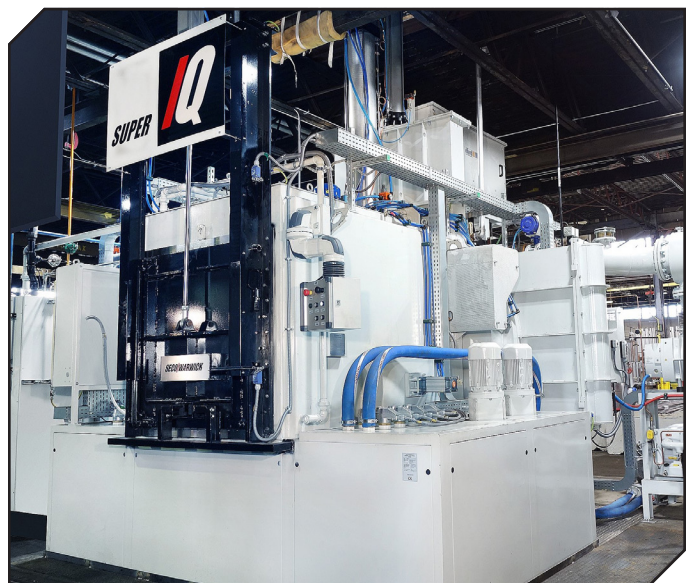
Figure 4 Clean integral quench carburizing furnace with no toxic gases and precision, high-volume carburizing for gears, shafts, and various other components.
