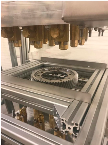
Figure 2—Test rig for WSpQ, providing a nozzle system positioned above and below the parts to be quenched.
