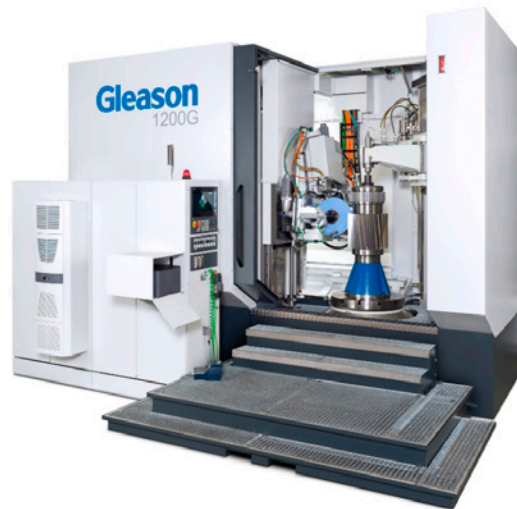
Figure 7—All Gleason profile grinding machines up to 6,000 mm in workpiece diameter feature the A(X) infeed-strategy software.
