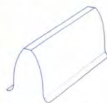
1 involute tooth profile without any modifications
