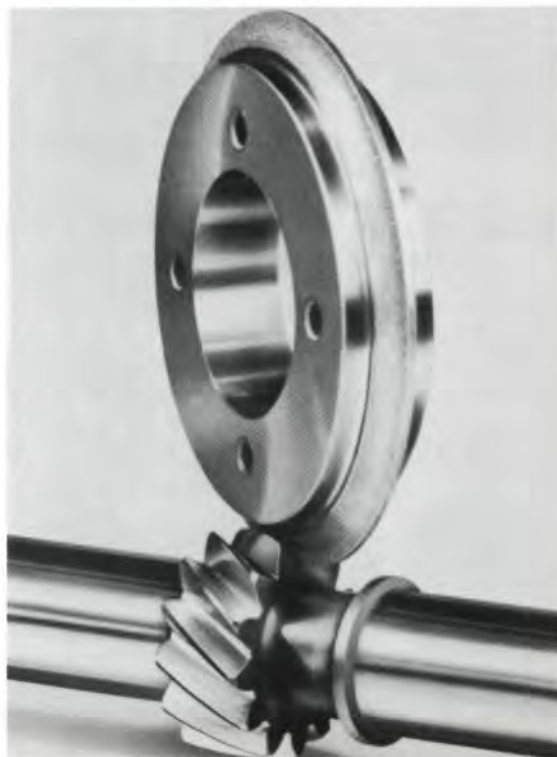
Fig. 22—A thin coating of CBN applied to a steel based wheel.
