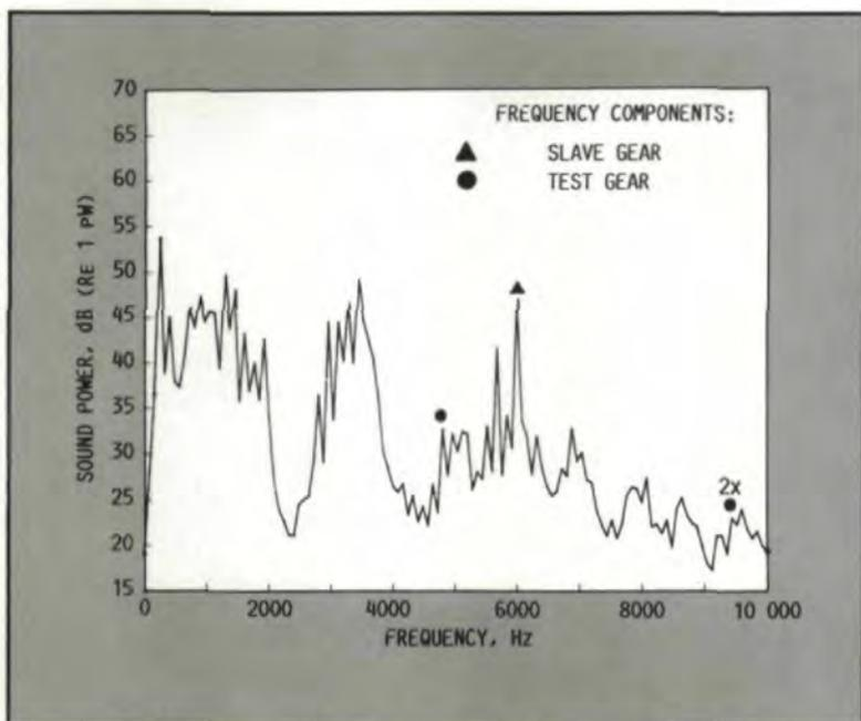
Fig. 7—Sound power for four planes investigated (conditions: standard gear, 10 160 RPM, 1615 N).
