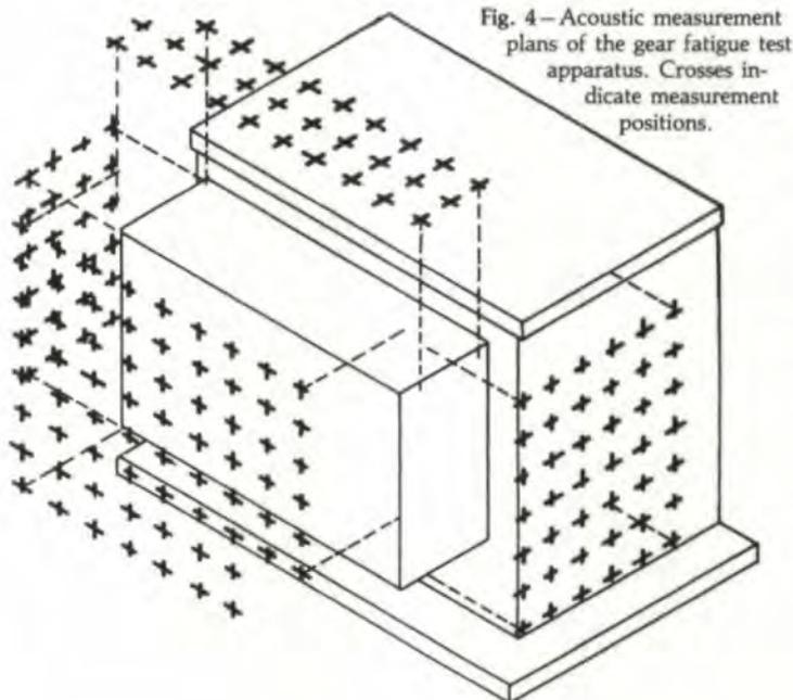
Fig. 4—Acoustic measurement plans of the gear fatigue test apparatus. Crosses indicate measurement positions.
