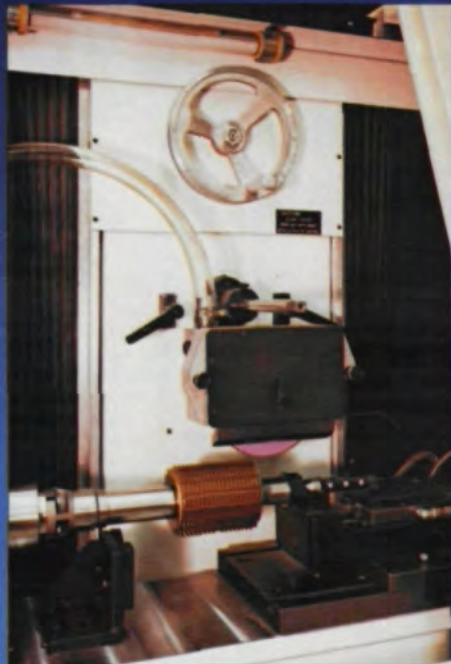
Lighted sharpening area is completely enclosed with sliding access door. (Grinding spindle assembly is easily accessible through sliding doors at rear of machine).
