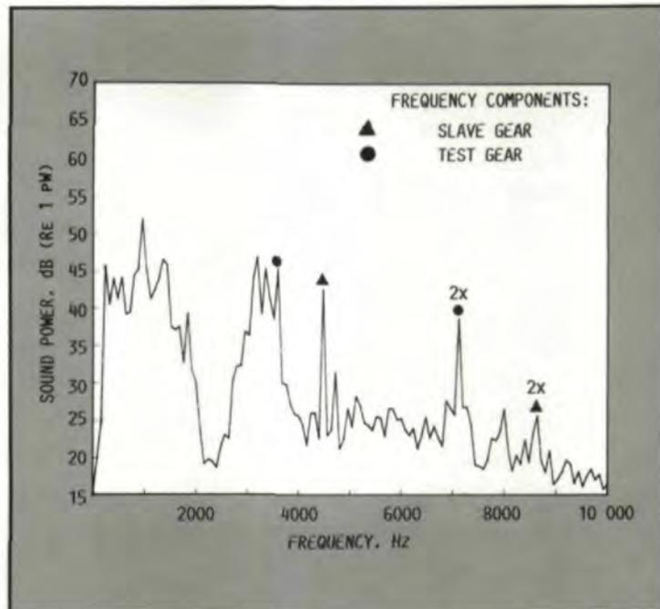
Fig. 8—Sound power for the four planes investigated (conditions: standard gears, 7470 RPM, 1615 N).
