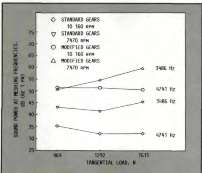
Fig. 11—Sound power versus mesh frequencies and loading.
