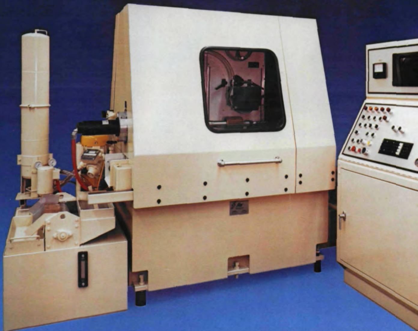
The new Star CNC horizontal hob sharpener is specially designed to bring the superior performance and longer life of Borazon® grinding wheels to this operation. The machine is capable of sharpening straight gash hobs up to 10"- diameter and 12"- long to AGMA "Class AA" tolerances.
