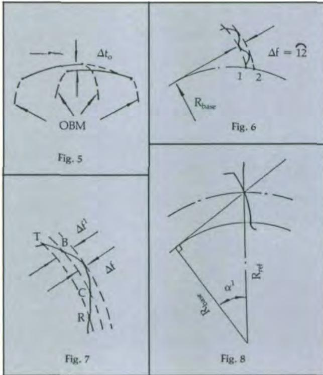
is defined as the profile error. (Fig. 6). If the BT/CR section is used for tip/root relief, then only the shape error of BC section will count. Tip/root relief should not be confused with profile error. As shown in Fig. 7, profile error is  $\Delta f$  instead of  $\Delta f'$ .
