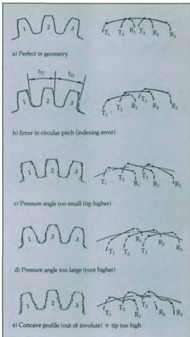
Fig. 2 - Geometric errors expressed on tester's record.
