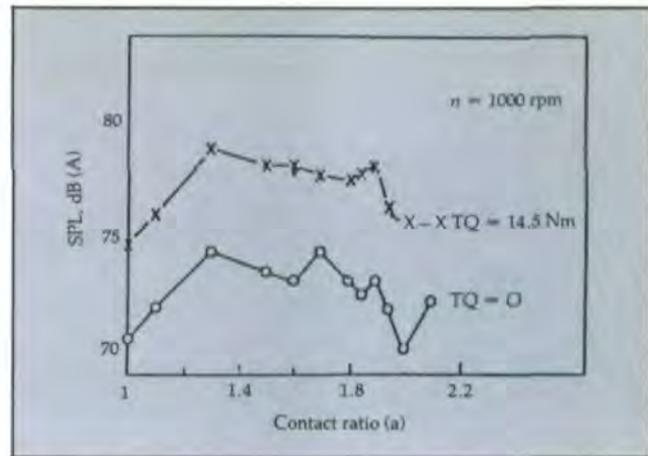
Fig. 17 - Relation between contact ratio and noise level
