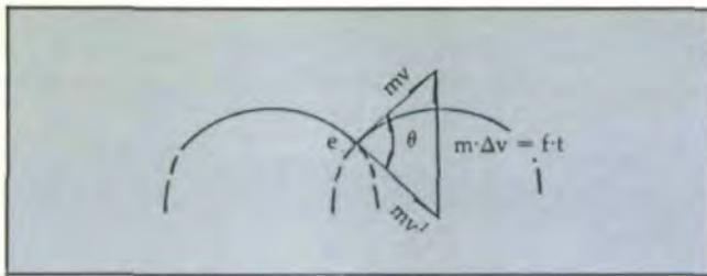
Fig. 4 - Vector diagram of change over impact.
