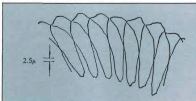
Fig. 15 – Tester's record of gear with convex profile
