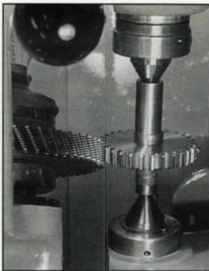
Fig. 2 - Crossed axes meshing of shaving cutter and work gear.
