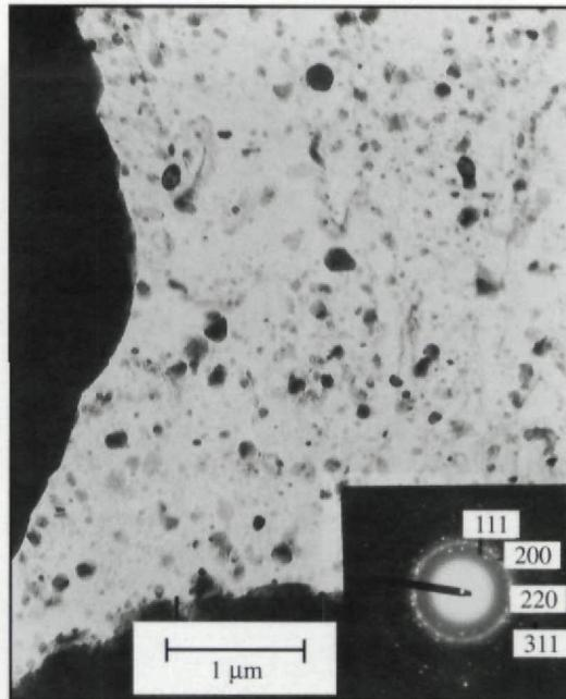
Fig. 4c — Microcarbides ( $Mo_2C$ ) precipitated by ausrolling.
