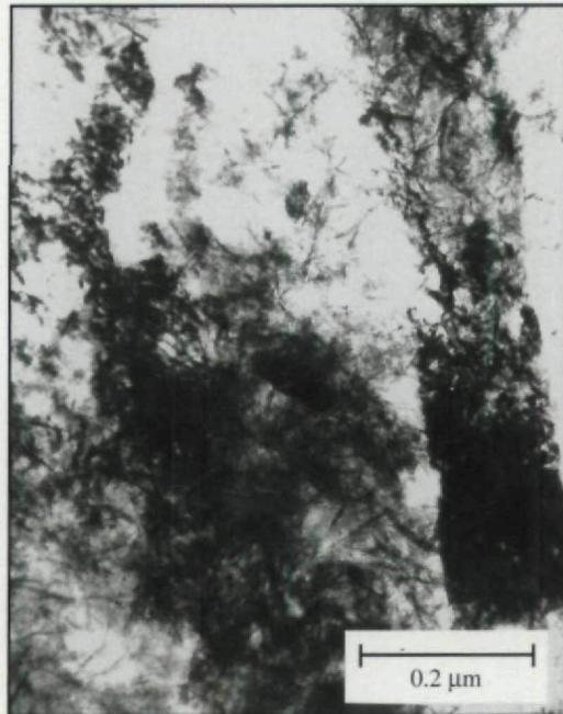
Fig. 4b — Ausrolled dislocations inherited by martensite.
