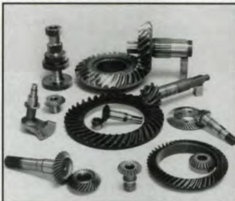
**Spiral & Straight Bevel Gear Manufacturing.**
