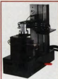
Modular gear blank fixture
