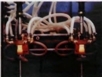
**ScanPak.** A versatile vertical scanner that allows the user to harden shaft-like parts from camshafts to hydraulic pistons, ScanPak is available in nine different configurations, in power ratings up to 800 KW, in frequencies to 50 KHz. Whether you need single spindle, dual spindle, or twin drive, there is a ScanPak exactly suited for you. ScanPak comes equipped with microprocessor-based machine control, integral heat station, and with spindle sizes up to 60".
