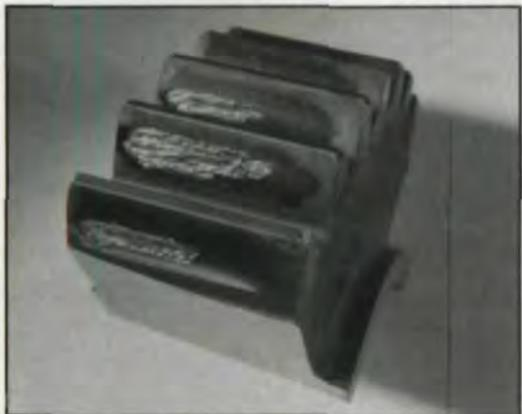
Fig. 2 — Pitting on the flanks of gear teeth.
