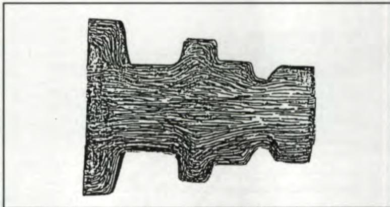
Fig. 1 — The correct distribution of fibers in a gear.
