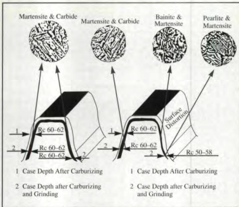
Fig. 7 — Results after graded hardening and oil quenching.
