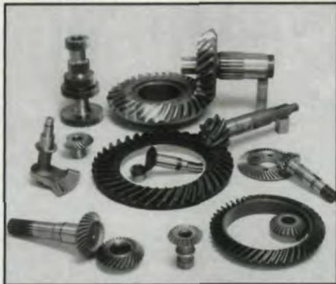
**Spiral & Straight Bevel Gear Manufacturing.**
