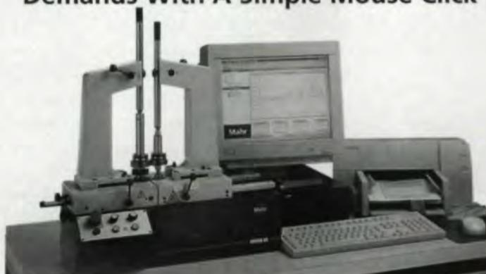
Yes, it's that easy to get accept/reject test results to ISO, AGMA and DIN standards with Mahr's new DF1 890 series double flank gear roll testers. Easy-to-use, Windows® '95-compatible WinGear® test and evaluation software lets you determine Total Composite, Tooth-to-Tooth and Radial Runout errors with a single mouse click.
