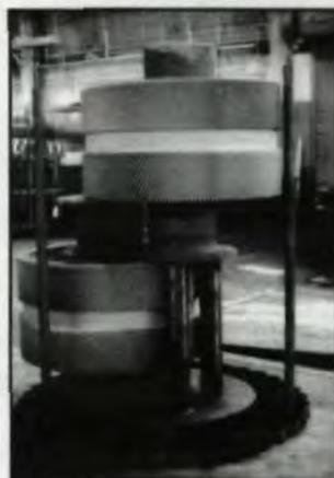
Two 137T, 5 D.P. gears just after nitriding. They will be used in a 13,000 HP marine drive.
