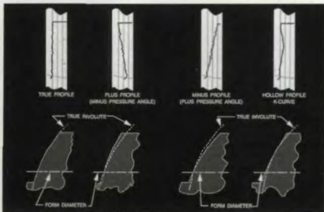
Fig. 15 — Typical profiles that can be ground on broaches.
