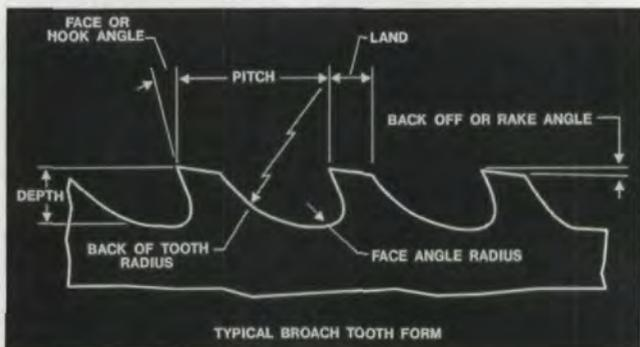
Fig. 2 — Parts of a broach tooth.
