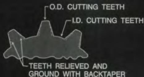
Fig. 7 — Concentricity between the inside and outside diameters.
