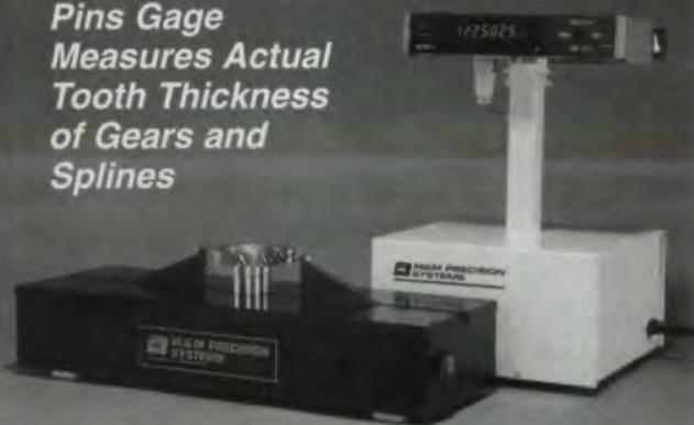
M & M Precision Systems now offers pitch diameter (tooth thickness/space width) Gaging Systems. Gear manufacturers can verify actual tooth or space thickness at the pitch diameter. A unique constant pressure gaging head assures accuracy over the full range of the gaging system. Both Automatic and Manual
