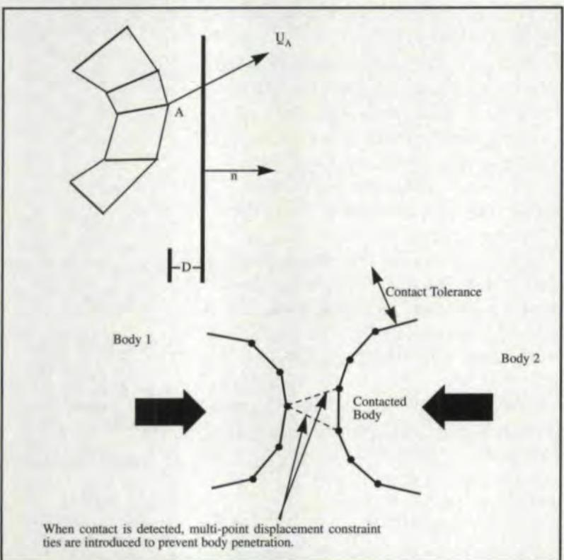
Fig. 6 — Non-penetrating constraints used in contact algorithm.
