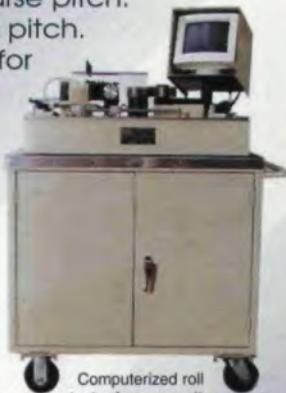
Computerized roll tester for composite and lead
