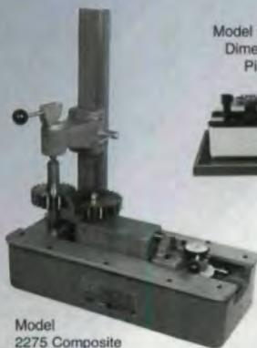
Model 2275 Composite Gear Roller
