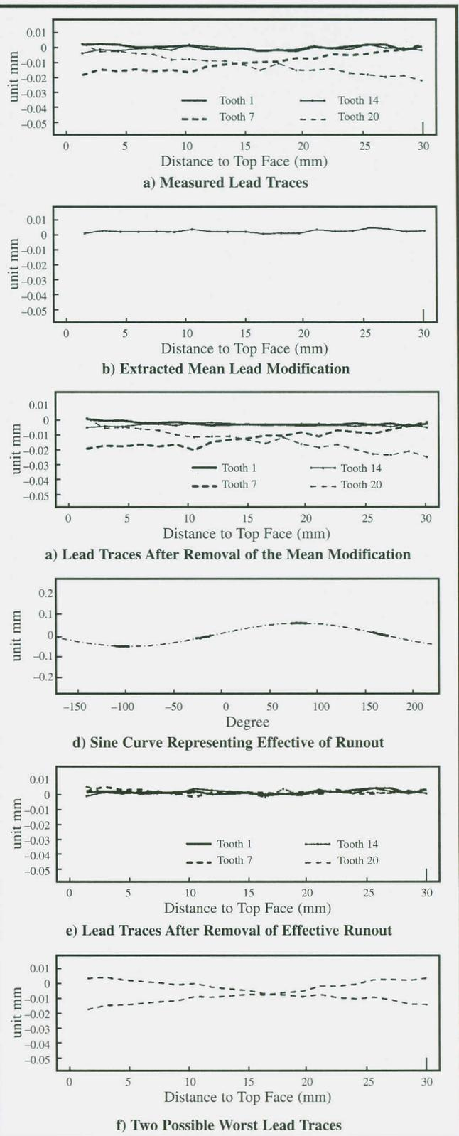
Fig. 4 - Example Gear Inspection: 4 teeth inspected; left flank; lead trace.
