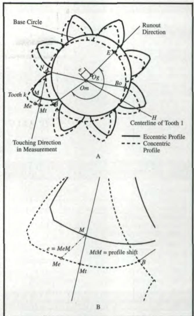
Fig. 1 - Profile Measurement on Eccentric Gear (left flank).
