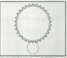
Fig. 3—Definining the tooth thickness and drawing the involute form.
