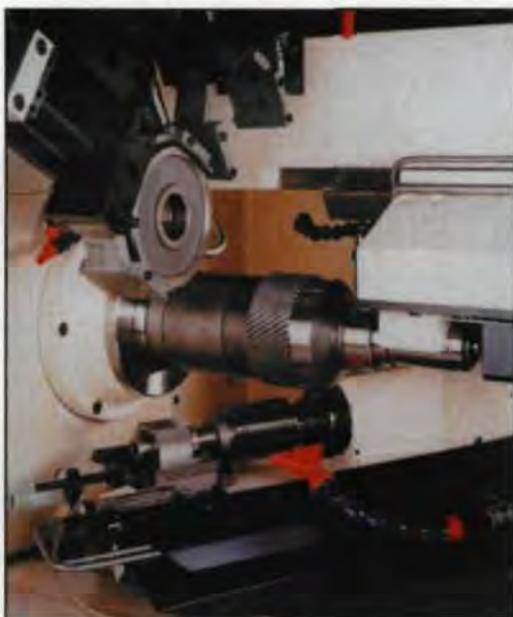
Figure 3—New CNC hobbing machine.
