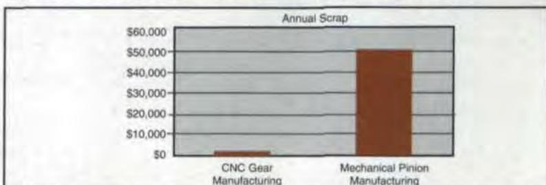
Figure 12—Comparison of annual scrap rates between CNC and mechanical manufacturing.
