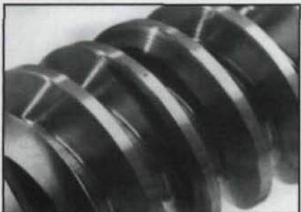
Fig. 3—Large score marks on a case-hardened worm.
