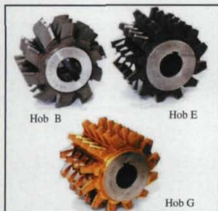
Figure 1—Carbide hobs used for cutting tests.
