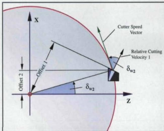
Figure 4—Blade with Offset 2 accommodates offset angle 1 by front face modification.
