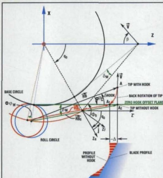
Figure 11—Epicyclic kinematics of two different blade types.
