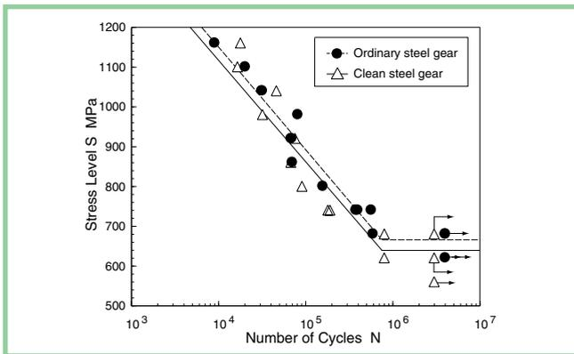
Figure 8—S-N curves in 4200 gears and 420C gears.
