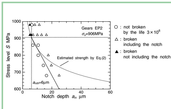
Figure 1—Strength of electropolished gear with a micronotch.
