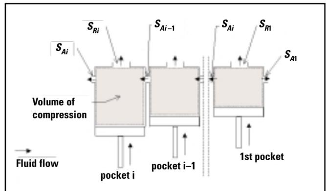
Figure 2—Discrete hydrodynamic model for helical gears.
