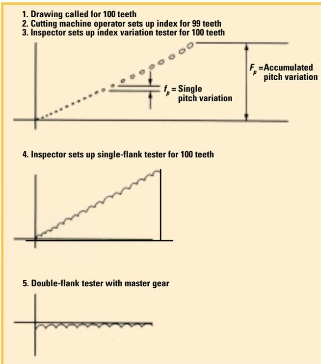
Figure 9—An extreme example to show the advantages of single-flank vs. double-flank composite tests.
