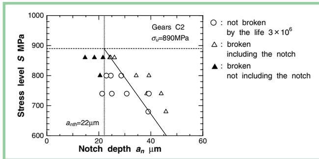
Figure 13—Strength of carburized gear with a micronotch.
