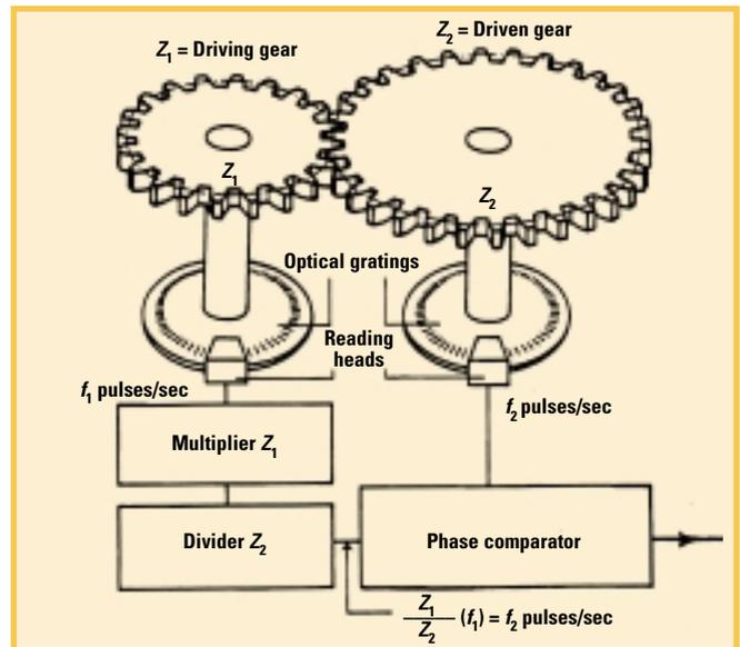
Figure 3—The principle of a single-flank measuring machine.
