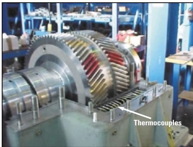
Figure 4—High speed test rig.
