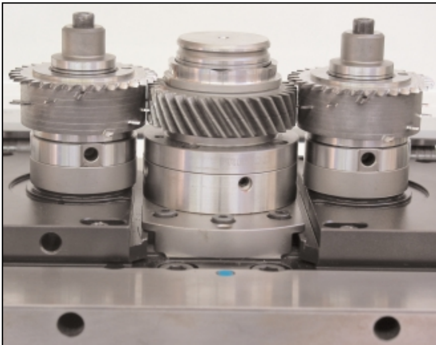
A helical gear is ready to have its involute profiles inspected by two "hedgehog master gears" on a RollScan machine. Licensed to Frenco GmbH, the RollScan can also use conventional master gears with whole teeth. The RollScan can inspect all of a helical gear's flanks and provide complete topographical information on them in less than two minutes.
