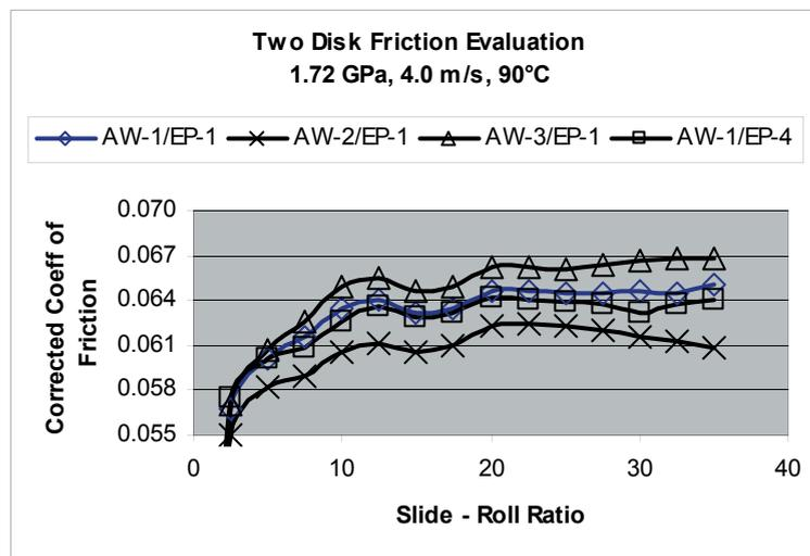
Figure 4—Two Disk Friction Response vs. Slide-Roll Ratio.
