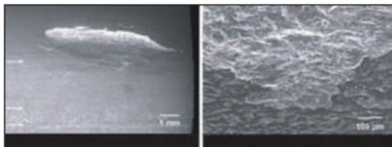
**Figure 4—SEM images of the No. 10 tooth of the tested pinion gear of the LH2 run using 7.5 cSt oil with an FZG Type GF-C micropitting gear. The area between the two outer arrows is the micropitting band.**
