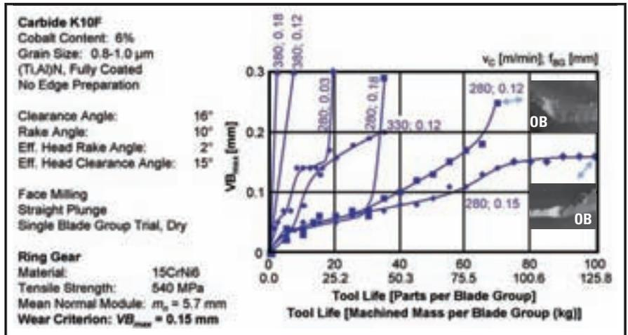
Figure 6—Wear charts of the cutting parameter variation.
