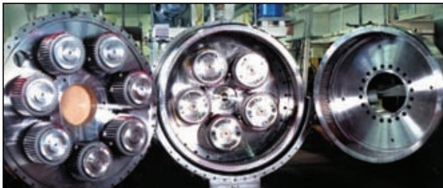
**Designed for Space, Weight—**Marine vessels often require more complicated gear arrangements, such as planetary gear systems, so their gearboxes meet space and weight restrictions. Such complicated gearboxes are common among many larger marine vessels. Photo courtesy of Maag Gear AG.
