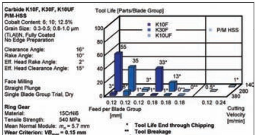
Figure 8—Tool life overview of the substrate variation.
