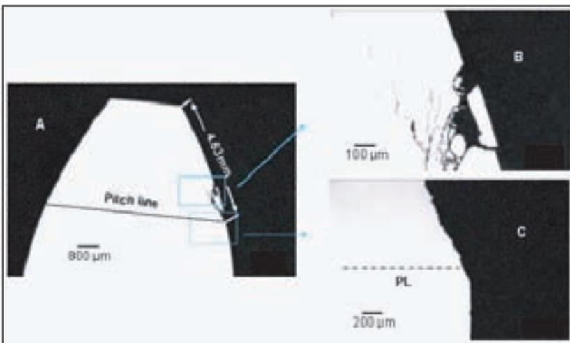
Figure 7—SEM image of a cross section through a spall on the 2nd tooth of the HH2 run. This test involves a 15 cSt oil and a micropitting gear.
