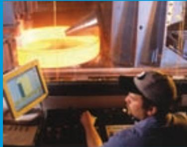
Rotek Incorporated offers a wide selection of seamless rolled rings in aluminum grades, and in carbon, stainless and alloy steels. All are certified, all are traceable. Rings can be produced in diameters from 18 inches to 160 inches, heights to 20 inches and weights to 8,000 pounds. Available profile configurations range from simple rectangular cross sections to complex shapes, including flanges, grooves and tapers.
