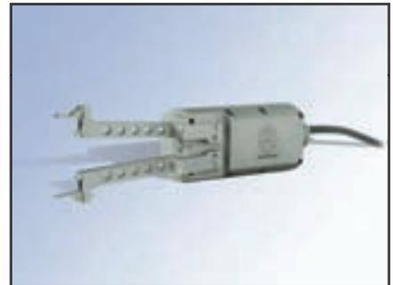
The gage is available in two sizes—the Model 50 with a 50 mm (1.97") body diameter for measuring inner diameters from 50 mm (1.97") up to 170 mm (6.69") and Model 70 with a 70 mm (2.75") body diameter for measuring inner diameters from 75 mm (2.95") up to 220 mm (8.66").
