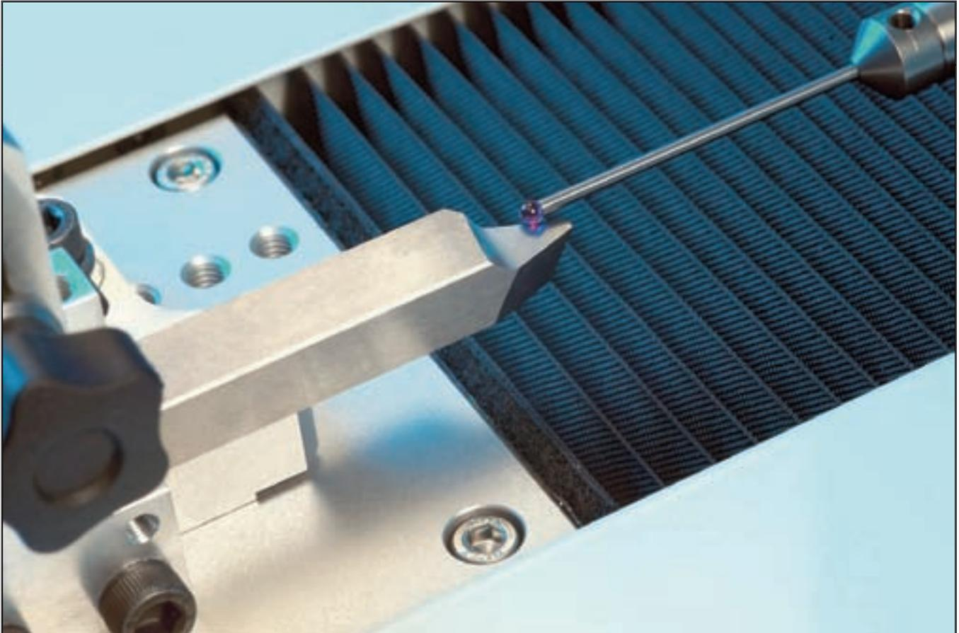
Meant for use on the shop floor, the Oerlikon BC 10 scan-measures stick blades via ruby-tipped probes, collecting large amounts of information—like 200 data points on a blade's curved cutting edge—to ensure it properly cuts spiral bevel and hypoid gears.
