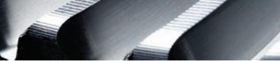
the amount of trials in the laboratory, since the number of required blanks is reduced by an order of magnitude. The blade wear is monitored over the tool life by measuring the wear land width or chipping size. Furthermore, all blades have been analyzed with a scanning electron microscope after the end of a trial. The end of tool life was defined as a maximum wear land width or chipping size of  $VB_{max} = 0.15$  mm.
