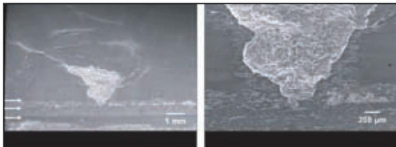
**Figure 2—SEM images of the No. 5 tooth of tested pinion gear of the LL2 run using the 7.5 cSt oil with an FZG Type PT-C pitting gear. The area between the two outer arrows is the micropitting band.**
