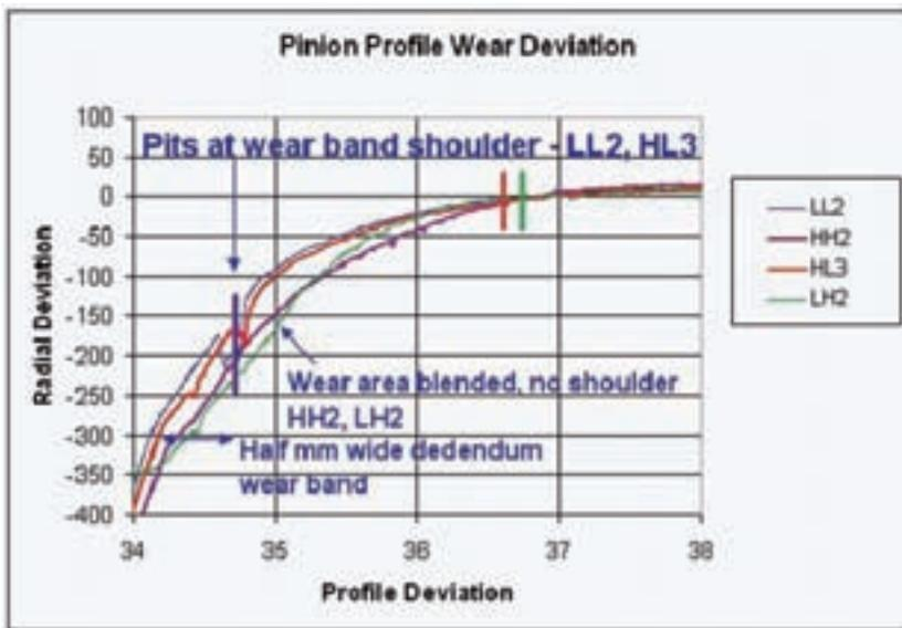
Figure 5—Wear-induced tooth profile deviation.
