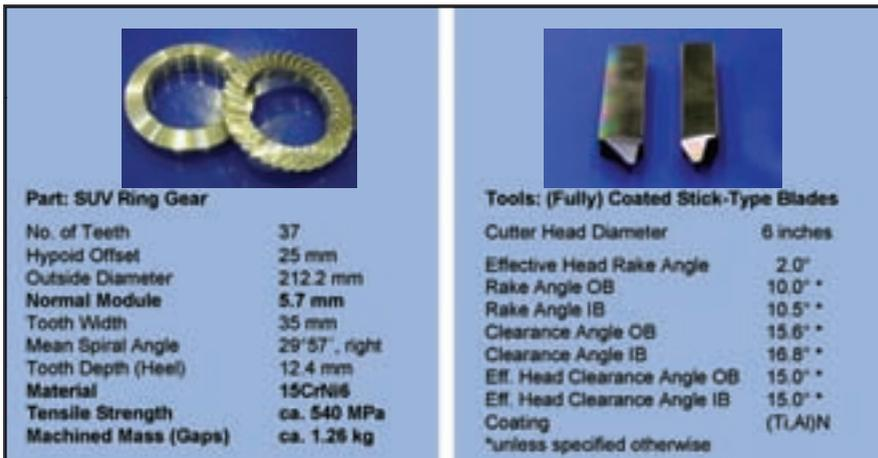
Figure 4—Trial workpiece and tool data.
