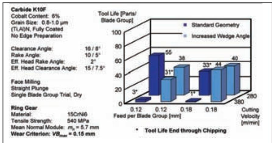
Figure 14—Comparison, standard geometry vs. increased wedge angle.
