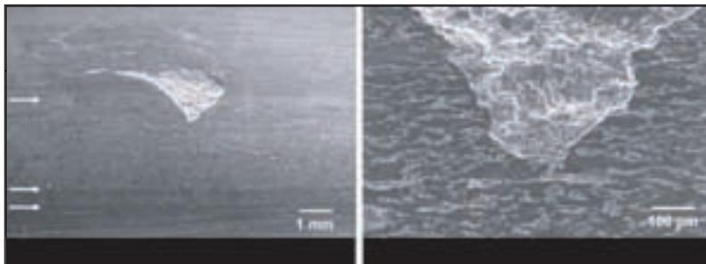
**Figure 3—SEM images of the No. 2 tooth of the tested pinion gear of the HH2 run using 15 cSt oil with an FZG Type GF-C micropitting gear. The area between the two outer arrows is the micropitting band.**
