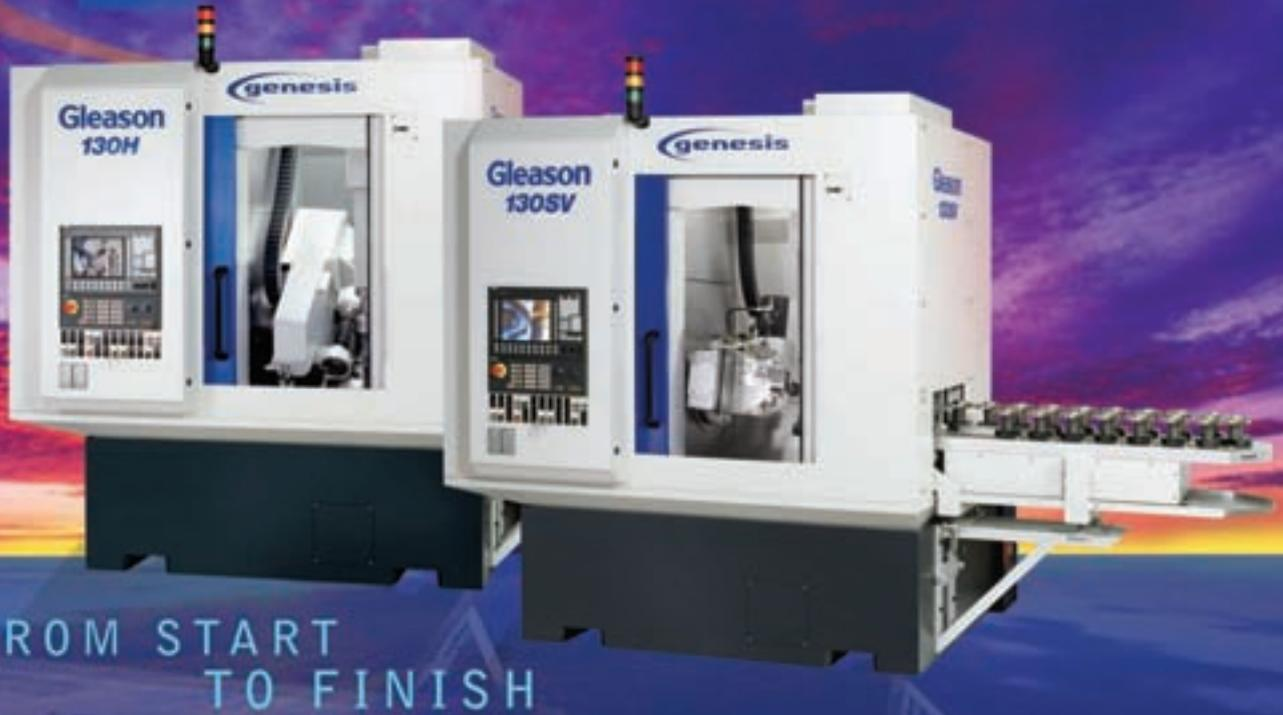
**T**he Genesis™ series of gear production machines is the next generation in gear production technology. The Genesis 130H Hobbing and 130SV Shaving Machines are available today to deliver more speed, greater precision and, above all, reduced cost in day-to-day operation for gears as large as 130 mm diameter.
