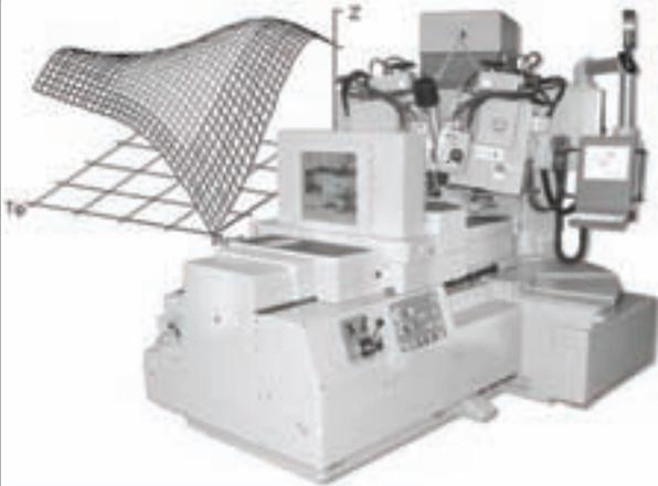
Advanced topological gear grinding, based on MAAG 0° grinding system.
