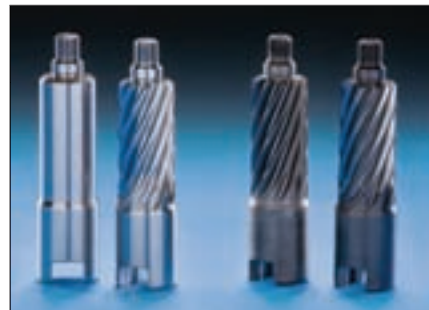
The K160 manufactures steering pinions by soft pre-hobbing and hard finish-hobbing (skiving) of the gearing.
