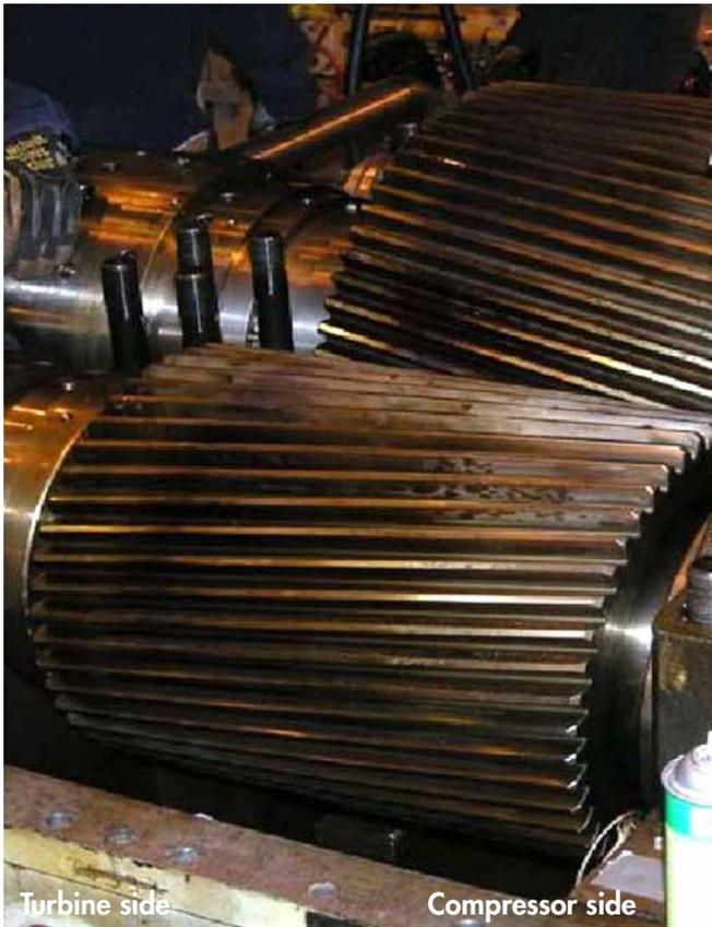
Figure 5—Varnish deposits on gear teeth.
