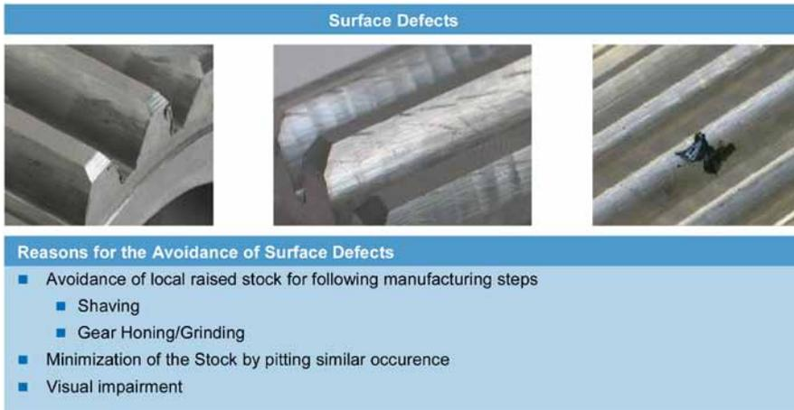
Figure 9—Surface defects.
