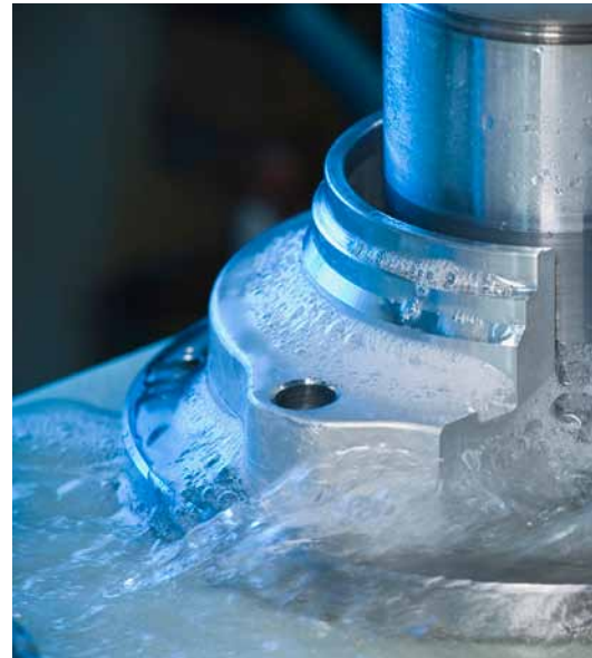
Precision Electro-Chemical Machining (PECM) is eliminating traditional steps in the machining process such as turning, milling and drilling (all photos courtesy of EMAG).
