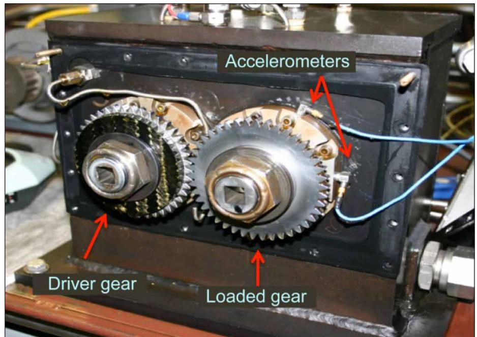
Figure 10 Test facility shown with cover removed.
