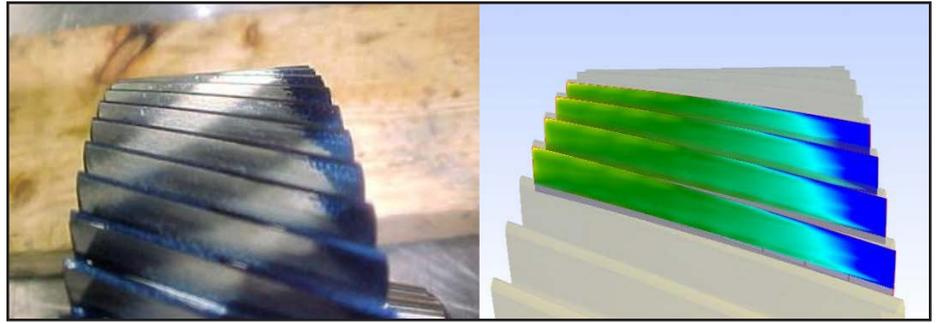
**Figure 5** Measured and simulated loaded contact patterns.
