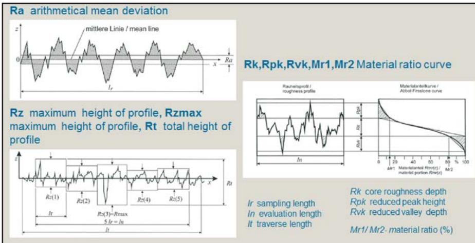
Figure 5 Roughness parameters according to DIN EN ISO 4287/13565.
