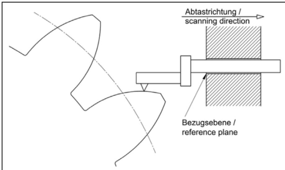
Figure 6 Skid less probing system with plane reference.
