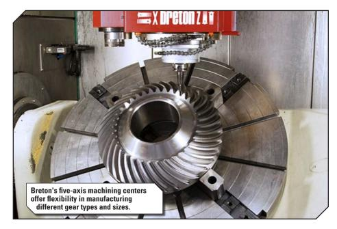
offering high machining performance when milling complex workpieces with five axes. The thermal symmetry of the machine structure and thermal stabilizing system ensure maximum machining precision when operational and production conditions vary.
