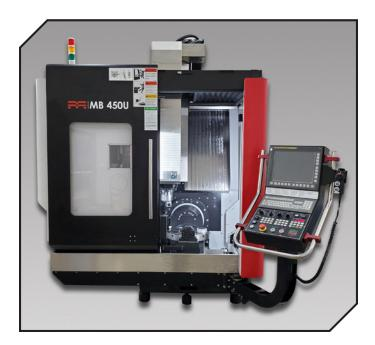
Due to the FANUC 31i-MB5 control, this machine is able to perform full five-axis precision machining of challenging parts, significantly reducing the need for multiple setups. Thanks to the control that is available exclusively to Methods, due to its partnership with FANUC, Methods Machining Centers are the only machines from Taiwan that can offer five-axis simultaneous.
