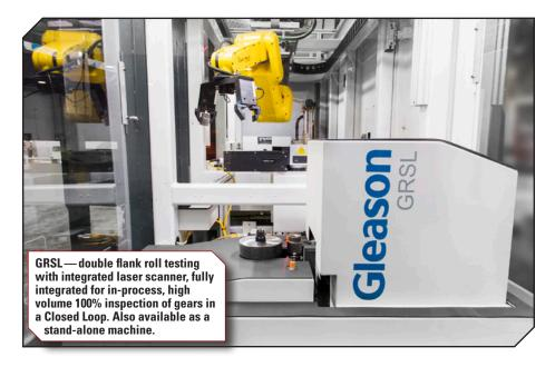
rejected. It is also possible to create extensive trend analyses of individual features and perform further gear noise analysis.
