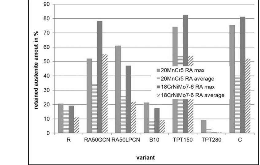
Figure 4 Comparison of the radiographically measured retained austenite amount, maximum and average values.
