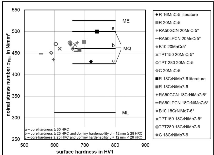
Figure 8 Classification of the determined allowable contact stress numbers for the examined variants in the standard strength diagram of ISO 6336 (Ref. 11) for case-hardened gears (\*reduced data points, additional values from literature [Ref. 16]).
