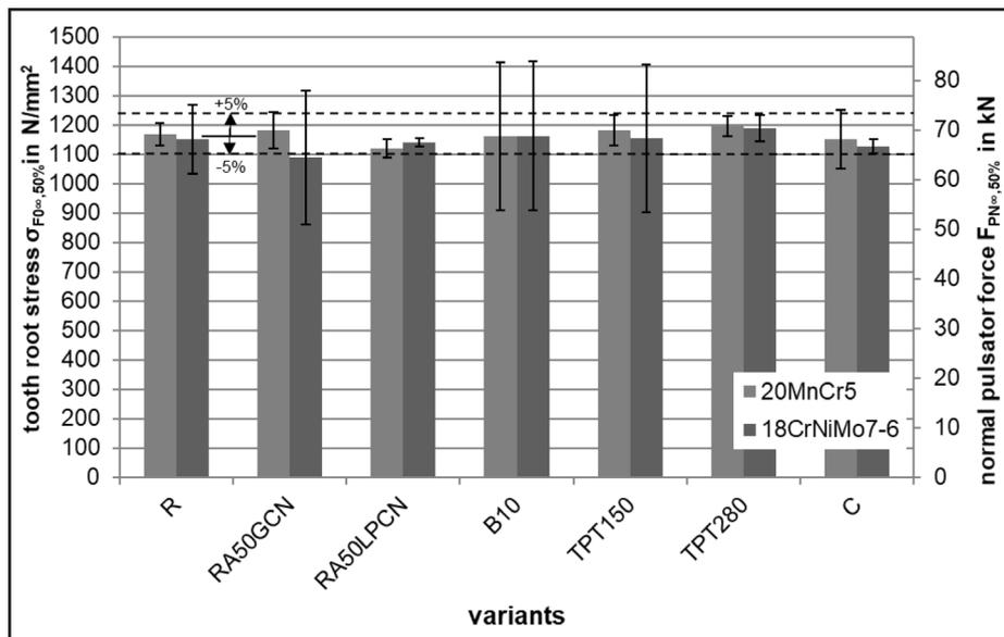
**Figure 5** Results of the nominal tooth root bending strength at a 50% failure probability ( $\sigma_{F0=,50\%}$ ) for all test variants.
